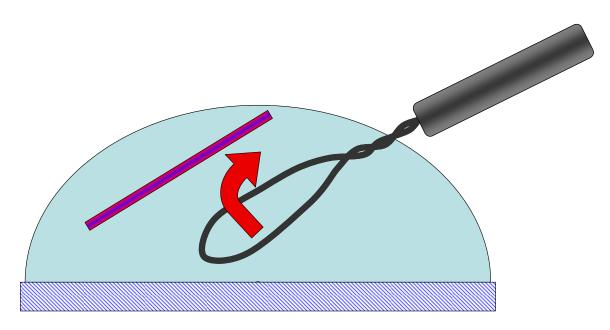
With one smooth motion lift the crystal up and back (towards the stem of the loop) so that the loop drags the crystal out of the mother liquor along its principal axis. Take care to avoid pushing the crystal upwards through the surface of the drop – that is an almost certain way to break the needle. In other terms, let the loop do the work of breaking the surface tension, not the crystal.
