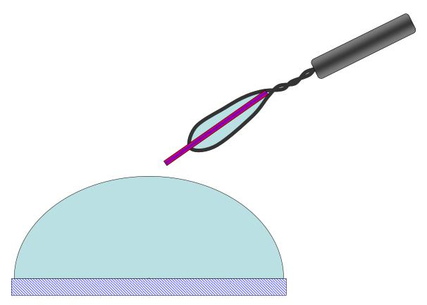
Assuming that you have adequate cryoprotectant in the drop, you should proceed with freezing (either in the cryo-stream or in liquid nitrogen, etc.). If you need to plunge the needle into cryoprotectant or oil, try to follow these directions in reverse – it is generally better to cryoprotect needles *in situ*, since repeated handling is likely to break them.
