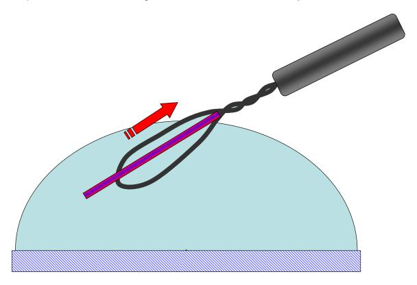
Pull the crystal all the way out, along its principal axis. If you have steady hands and the crystal is not excessively fragile, this should result in the needle selfaligning in the loop as shown below:
