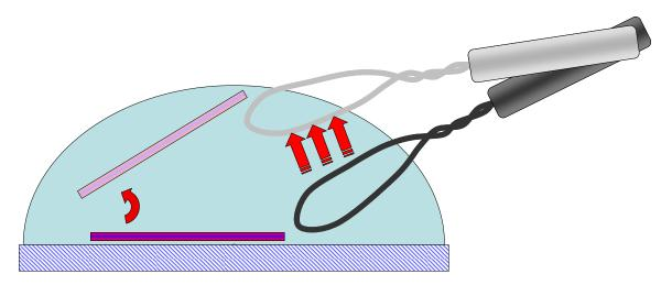
After the crystal is properly positioned, quickly place the loop under the crystal and align the principal axis of the loop with that of the crystal.
